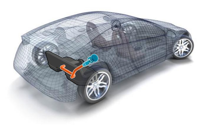
Ensure safe fuel handling by choosing Premix's electrically conductive HDPE compounds for fuel filler systems (FFS); heads, necks and pipes. Refueling generates static electricity in fuel filler system. It is caused by the friction between flowing gasoline and FFS's plastic surface. This static electricity might lead to gasoline ignition.
